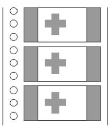
Now take into account that the design may have hundreds of these same part types in all four rotations on front and back. And then realize that, although this component is always 270° off, other polarized component types may only be 90° off, some others 180° and some may accidentally match. To the casual observer looking through the data file, the rotations would appear completely random! At this point, the rotations portion of the data file is virtually unusable.
