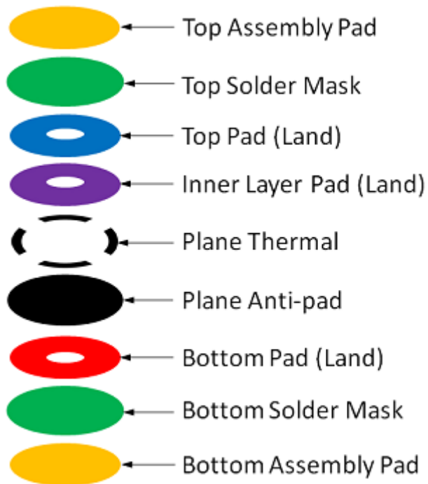
Figure 1. Plated through-hole padstack.
