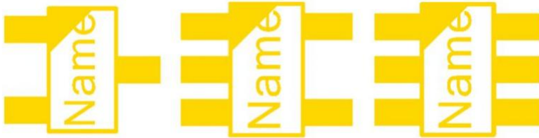
Figure 9. Silkscreen outlines for the various SOT component families.
