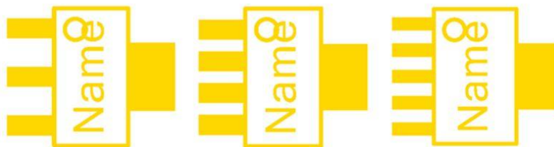
Figure 8: Assembly outlines for 4-, 5- and 6-pin SOT223.
