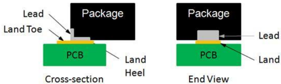
Figure 4. Side view of the QFN.
