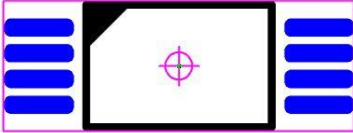
Figure 5. Enterprise CAD tool placement courtyard.
