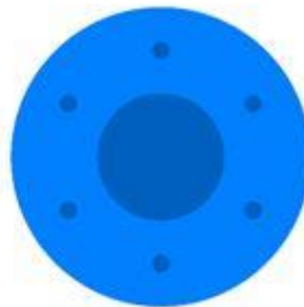
Figure 3. A supported mounting hole with vias.
