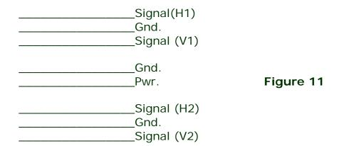
This is basically an eight-layer version of Fig. 7. It has all the advantages listed for Fig. 7, plus a tightly coupled power-ground plane pair in the center.
