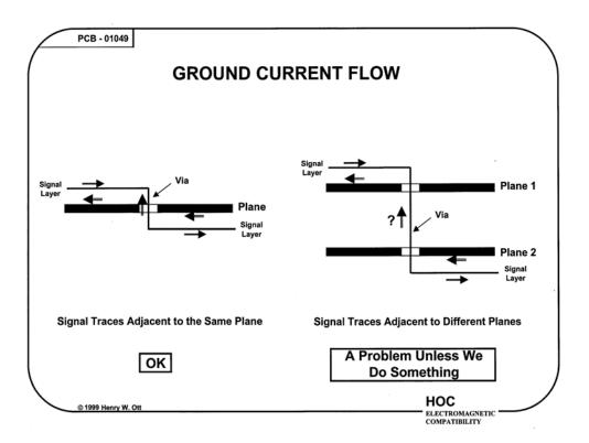
**Note**, that if the two reference planes are of the same type (either both power, or both ground) you can put a via (ground to ground or power to power) instead of a capacitor immediately adjacent to the signal via. This is a much better solution than using a capacitor to connect the planes together, since the added inductance in the return path will be considerably less.
