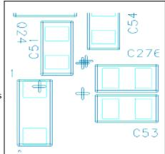
Another point that might be helpful to manufacturers would be to have the *shape* of the polarity mark be consistent. For example, I have seen filled circles, hollow circles, diagonal lines across corners, double lines and the number "1" on integrated circuits (ICs). Plus signs, curved lines, bold lines and the letter "C" or "K" have been on various types of diodes, many of which cannot be seen after the component is installed. Using marks consistently will help everyone involved.
