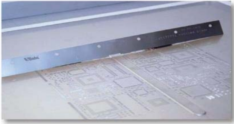
Figure 13: 3-D electroform stencil with notched e-blade.
